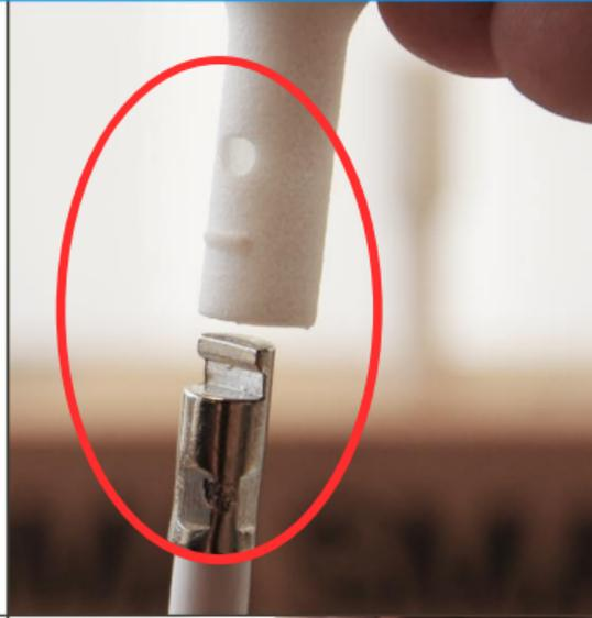
hold the cable with one hand and push the connector plug all the way in.
