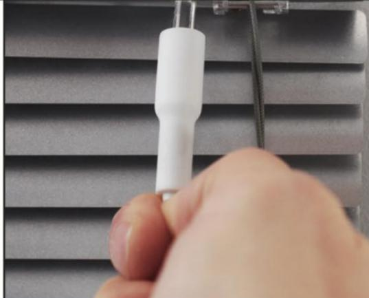
Once you have the right connector plug its time to attach it to Tilt Flex cable.
