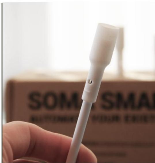
Pull the connector straight from the flex cable
